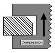
During the power stroke, the ring is sealed against the wall and the ring land by the pressure of expanding The same applies to the gasses. compression stroke though to a lesser degree. A worn ring will not seal as well as one that is within specifications. A poor seal does not directly result in oil transfer into the combustion chamber. It will result in a loss of crankcase vacuum. lower power and hard
