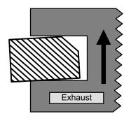
starting. The pressure that has leaked past is now in the crankcase wreaking havoc with the breather system and doing nothing to help put power to the PTO.
