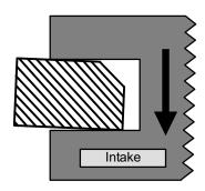
Although there are several issues that can cause or increase smoke from the exhaust, engine wear is the most common. Many people believe that wear allows oil to pass by the area of contact between the ring and the wall. This is to some degree true, but it is not the main avenue.
